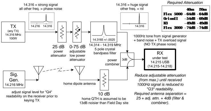
Final step is to design the antennas to produce more than the larger of the 2 required separations (in dB) for the tested TX/RX pair.
